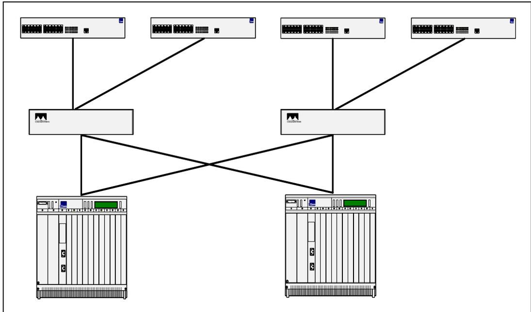
Figure 3-3 Star topology in an Ethernet network
